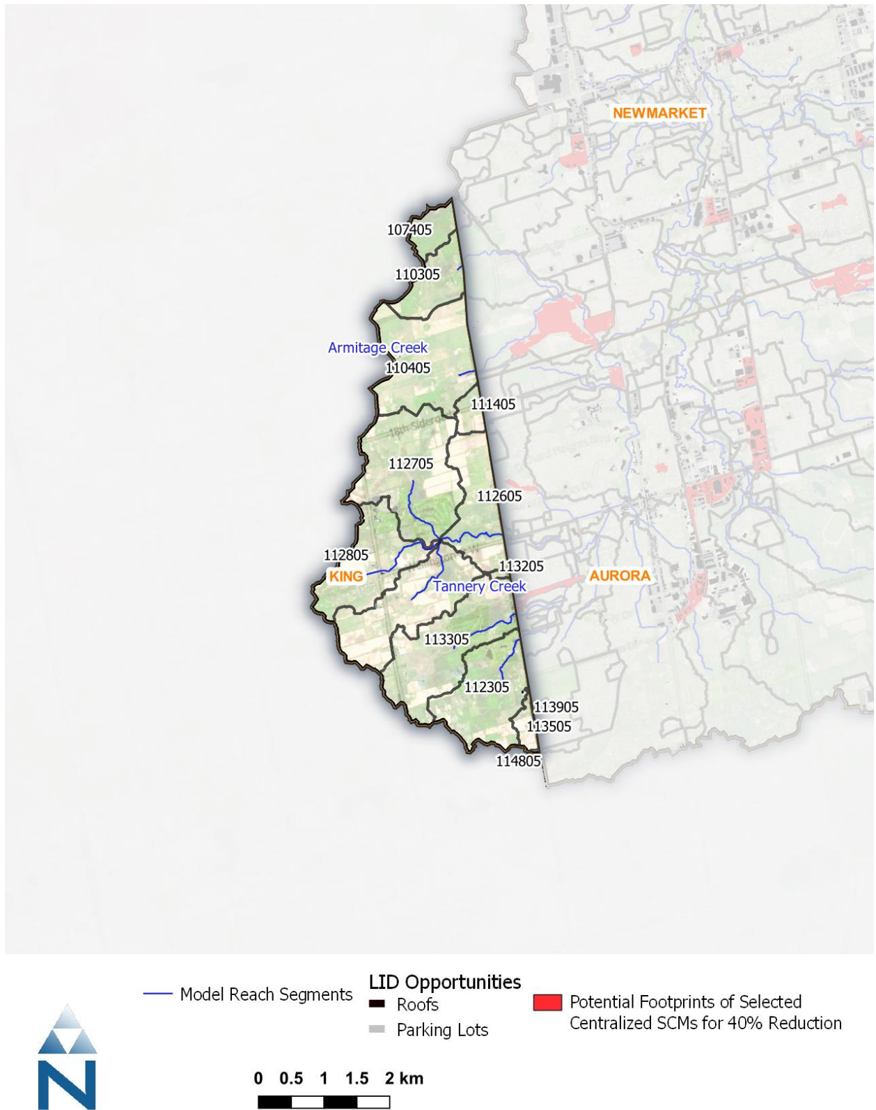
Figure 6. SCM footprint locations in King to achieve basinwide 40% TP reduction at Holland Landing.
