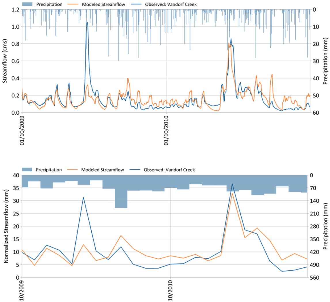
Figure C-7. Simulated vs. observed daily (top) and monthly (bottom) streamflow comparisons at Vandorf Creek (Station ID: Vandorf).
