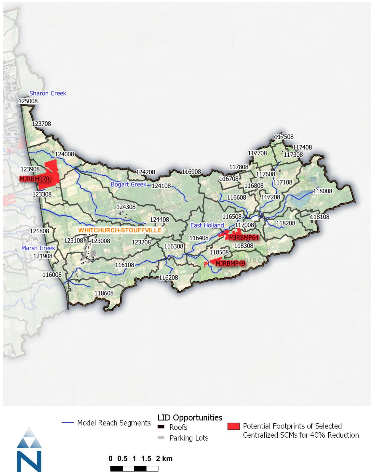
Figure 10. SCM footprint locations in Whitchurch-Stouffville to achieve basinwide 40% TP reduction at Holland Landing.
