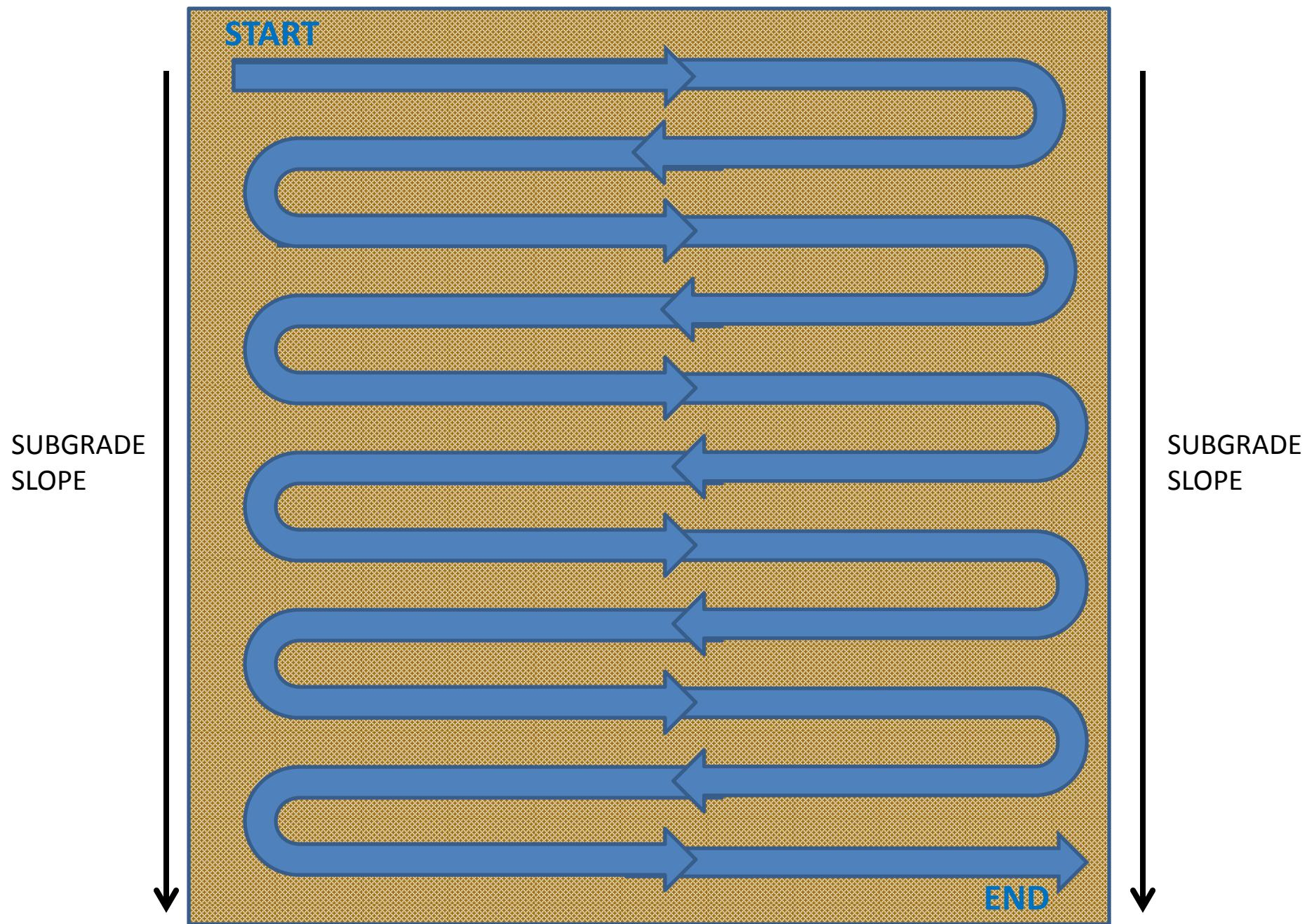
SUBSOIL SCARIFICATION PATTERN BY SOIL RIPPING USING EXCAVATOR OR BACK HOE
