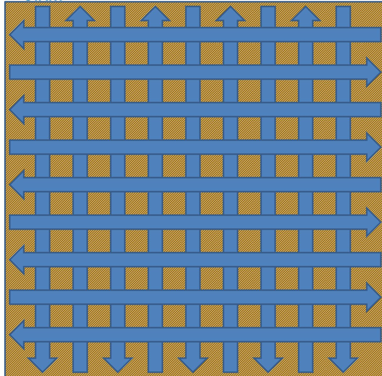
SUBSOIL SCARIFICATION PATTERN BY SOIL RIPPING OR TRENCHING PERPENDICULAR TO SUBGRADE SLOPE
