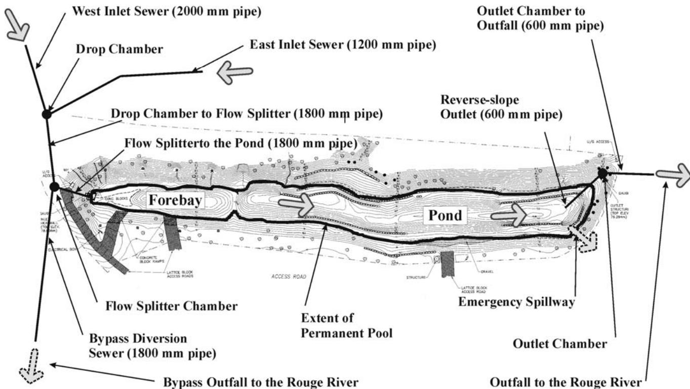
**Figure 1:** Rouge stormwater management pond
